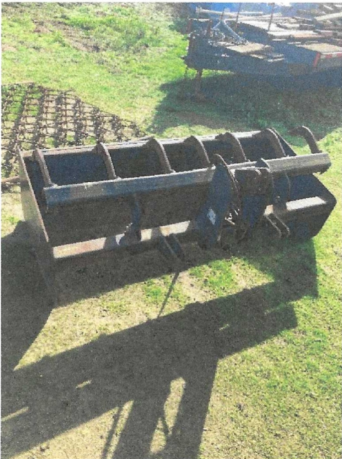
Box (Gannon) Scraper with Rippers
